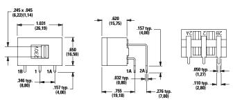
**Available with:** All models with 08 termination **PC Mounting:** PC mount, side actuated.
