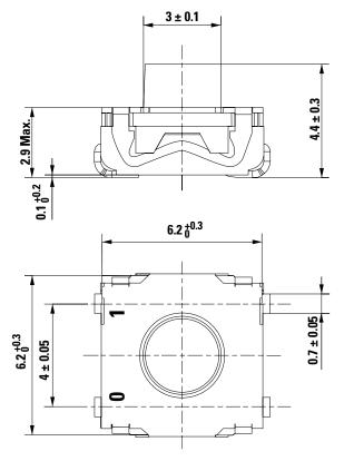
KSC7 Series Sealed Tactile Switch for SMT 6.2 x 6.2 mm, with 4.4 mm Height Soft Actuator
